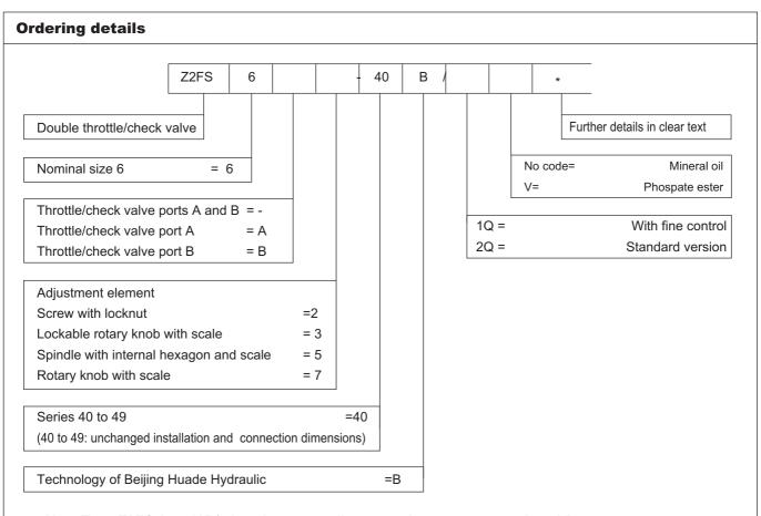
Note:Type Z2FS 6-...-40B/...has the same adjustment elements on ports A and B
