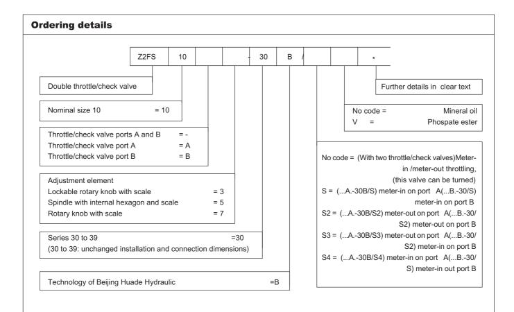
Note:Type Z2FS 10-..-30B/..has the same adjustment elements on ports A and B!
